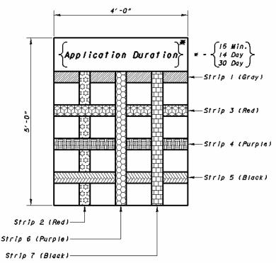
G. Apply permanent marker lines to the coated concrete next to, not on, the paint stripes.
